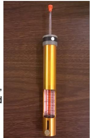
Figure 1: Sample of standard length inserted into spinner and properly positioned in depth gauge.
