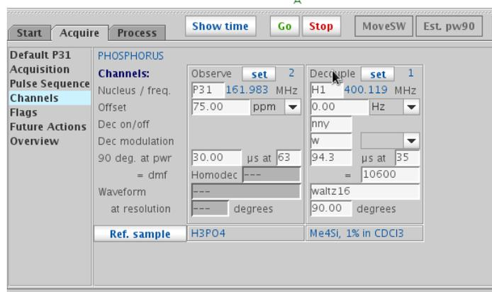
Figure 1: Customizing the centre of the phosphorus dimension of the phosphorus HMBC. Set the phosphorus offset to be close to the expected chemical shift of phosphorus for better results.
