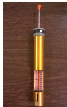
Figure 2: Sample adjusted properly in the depth gauge.
